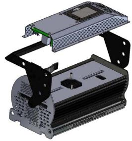
13. Tighten four self tap screws ST3.5 at four locations with screwdriver #4 to a torque of 5.5 lb-in.
